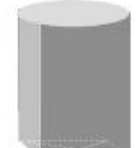
"O" – formed from circular woven fabric (the bottom can be as a sewn square canvas, as well as formed from soft container's body).
